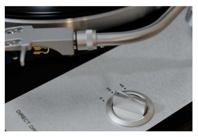
The TN-4D has a brushless direct drive with feedback control and two speeds of 33.3 and 45 rpm, therefore there is no platter bearing. This policy is meant to prevent or reduce "cogging." "Cogging" is a jerking sensation that might occur with direct drive. The die-cast aluminum platter is then placed on the DC motor's axis. The TN-4D lacks an automated start/stop mechanism that lifts the tonearm at the end of a record to protect the cartridge. You must assist in this situation.
